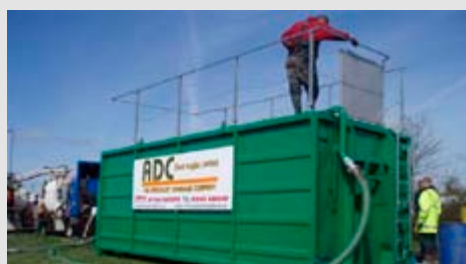
The AVC Dewatering container.
